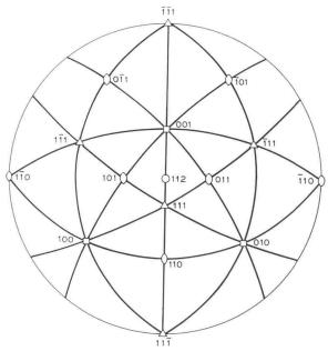
Fig. 1. Standard (112) stereographic projection for a cubic crystal.
